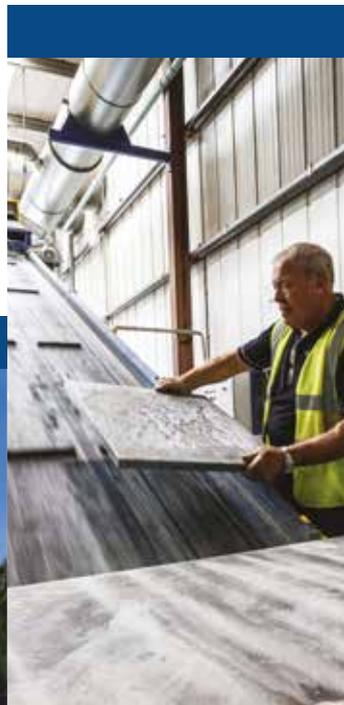
As part of our recycling scheme, we can offer a service that receives site returns of off-cut Kingspan panels from our customers. The steel and chipboard in the off-cuts are then separated in a £250,000 shredder (pictured) at our Hull site and then recycled so they can be put back into the manufacturing process.
